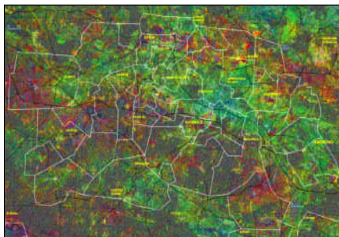
Fig 11: Differential SAR interferogram (D-InSAR) used for analysis of the patches of ground subsidence caused by underground coal mining during the period 04 Oct., 1992 to 08 Nov., 1992 in Upper Silesia, Poland.
