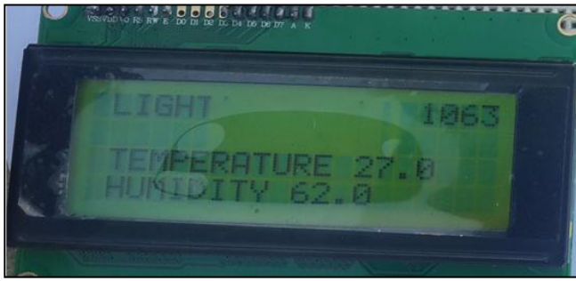
Fig 12: Display of real time Light Intensity, Temperature and Humidity
