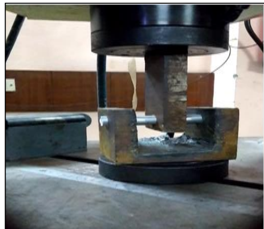
Fig 5: Setup up off shear test
