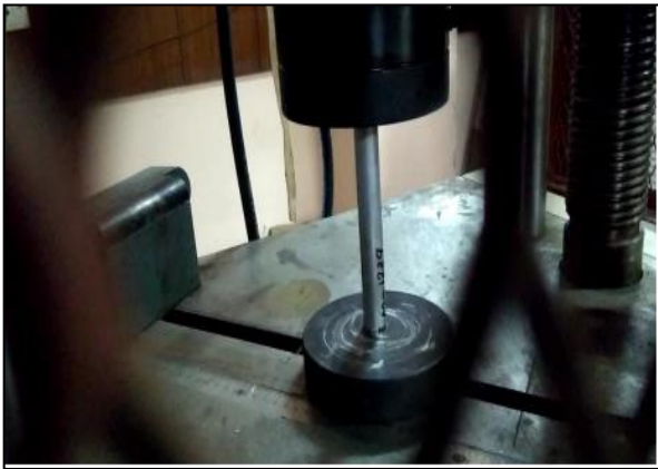
Fig 1: Setup off compressive test
